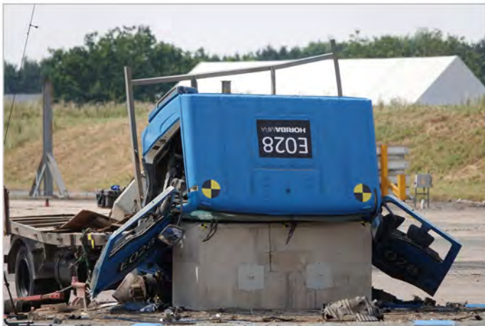
Post-impact: the cab is arrested on the block with no penetration of the barrier
