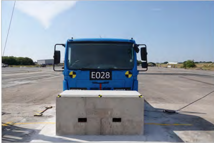
Fix Block 50 positioned ahead of a 7.5 tonne MAN rigid test vehicle prior to impact
