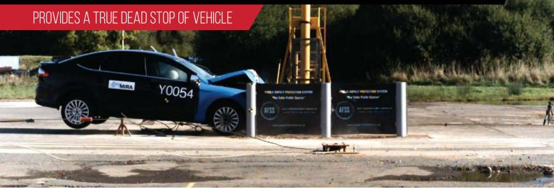
PUBLIC IMPACT PROTECTION SYSTEM (PIPS) is revolutionary in providing a true dead stop from the vehicle front bumper, with NO part of the vehicle projecting forward beyond the product face and into the safe zone on both the independent tests.
