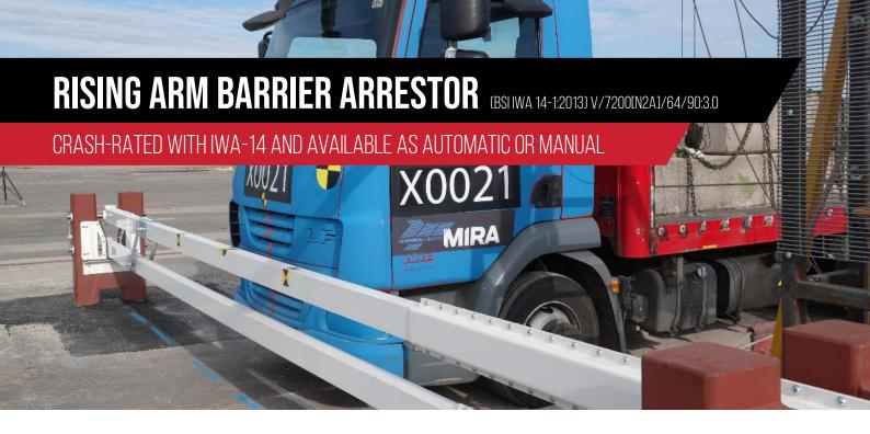
The Eagle Rising Arm Barrier is the latest addition to the Eagle's portfolio of crash tested products. Tested at a clear opening of 7.1m it meets our secure before impact (SBI) criteria utilising an au-tomatic or manual locking pin on the closing portal.
