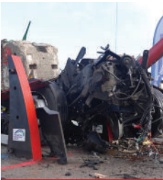
CITY PROTECT M50 after the crash test
