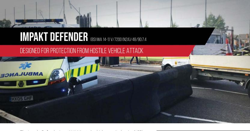
The Impakt Defender is an IWA14 rated vehicle security barrier (VSB) designed to protect people, buildings and infrastructure from hostile vehicle attack. Requiring no foundations, the surface mounted system can be rapidly deployed as a temporary or permanent security measure, as part of a robust hostile vehicle mitigation (HVM) strategy.
