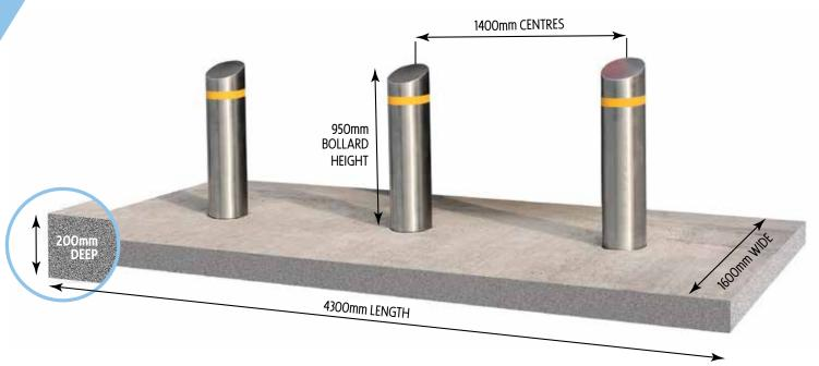
FOUNDATION SIZE FOR THREE BOLLARD RUN
